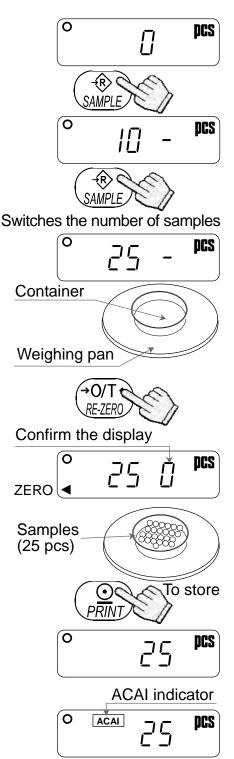
9. The ACAI indicator will blink and the balance re-calculates the unit weight. Do not touch the balance or samples on the pan until the ACAI indicator turns off.
